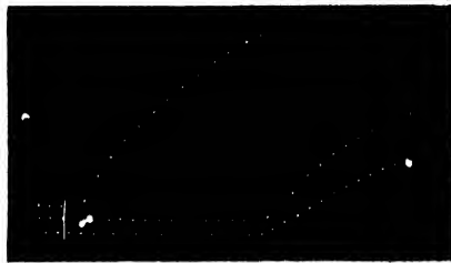
Fig. 119. Determination of velocity of Transmission of Excitation in petiole of Mimosa . Two lower records are in response to indirect stimulation applied at a distance of 30 mm.; upper record of response to direct stimulation gives the latent period. Recorder tuned to 10 V per second.
